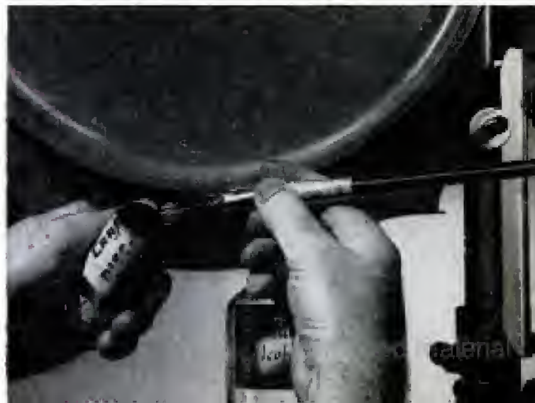
Above, use cement to prevent slipping of either flat or V-belts. Apply to the sides of a V-belt as indicated. Below, loose tires on bandsaw wheels are easily recemented in place by applying cement diluted with alcohol. Remove excess cement with turpentine
